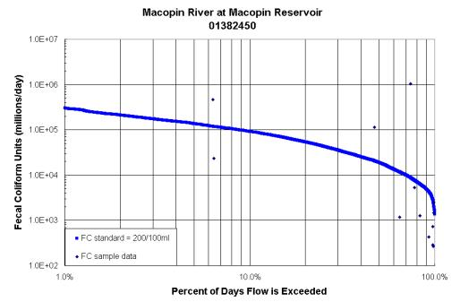
Load Duration Curve for Macopin River at Macopin Reservoir. Fecal coliform data from USGS station # 01382450 during the period 10/1997 through 8/2000. Water years 1970-2000 from USGS station # 01388500 (Pompton River at Pompton Plains NJ) were used in generating the FC standard curve.
