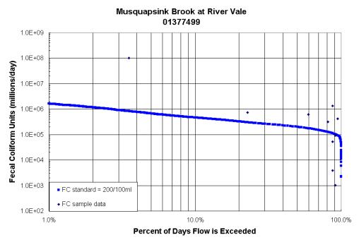
Load Duration Curve for Musquapsink Brook at River Vale. Fecal coliform data from USGS station # 01377499 during the period 7/13/99 through 9/7/00. Water years 1970-2000 from USGS station # 01377499 (Musquapsink Brook at River Vale) were used in generating the FC standard curve.
