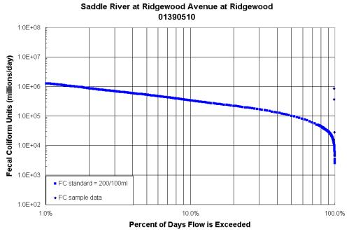
Load Duration Curve for Saddle River at Ridgewood Avenue at Ridgewood. Fecal coliform data from USGS station # 01390510 during the period 7/13/99 through 8/9/99. Water years 1970-2001 from USGS station # 01390500 (Saddle River at Ridgewood) were used in generating the FC standard curve.
