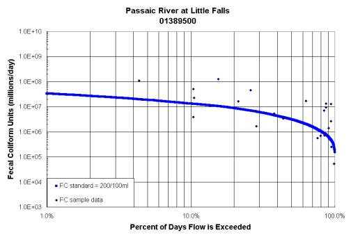
Load Duration Curve for the Passaic River at Little Falls. Fecal coliform data from USGS station # 01389500 during the period 2/18/94 through 9/23/98. Water years 1970-2000 from USGS station # 01389500 (Passaic River at Little Falls) were used in generating the FC standard curve.
