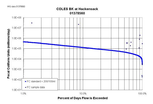
Load Duration Curve for the COLES BK at Hackensack. Fecal coliform data from USGS station # 01378560 during the period 11/5/97 through 8/23/00. Water years 1970-2001 from USGS station # 01391500 (Saddle River at Lodi) were used in generating the FC standard
