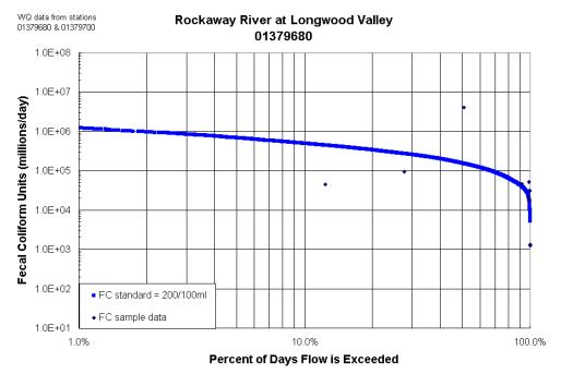
Load Duration Curve for Rockaway River at Longwood Valley. Fecal coliform data from USGS station # 01379680 & 01379700 during the period 1/27/97 through 9/2/99. Water years 1970-2000 from USGS station # 01380500 (Rockaway River above Reservoir at Boonton) were used in generating the FC standard curve.
