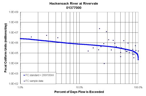
Load Duration Curve for the Hackensack River at Rivervale. Fecal coliform data from USGS station # 01377000 during the period 2/17/94 through 8/3/00. Water years 1970-2000 from USGS station # 01377000 (Hackensack River at Rivervale) were used in generating the FC standard curve.
