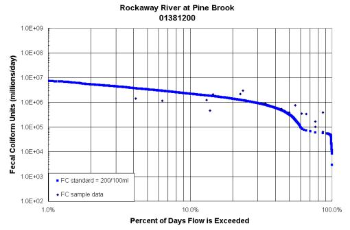
Load Duration Curve for the Rockaway R at Pine Brook. Fecal coliform data from USGS station # 01381200 during the period 10/1997 through 8/2000. Water years 1970-2000 from USGS station # 01381000 (Rockaway River below Reservoir at Boonton, NJ) were used in generating the FC standard curve.
