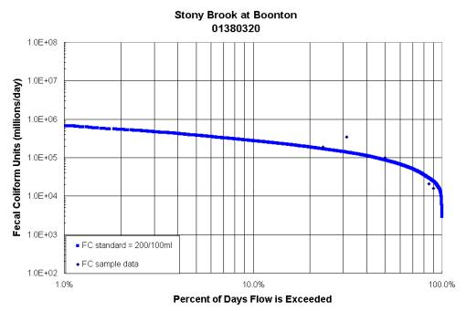
Load Duration Curve for Stony Brook At Boonton. Fecal coliform data from USGS station # 01380320 during the period 12/13/99 through 9/7/00. Water years 1970-2000 from USGS station # 01380500 (Rockaway River above Reservoir at Boonton) were used in generating the FC standard curve.
