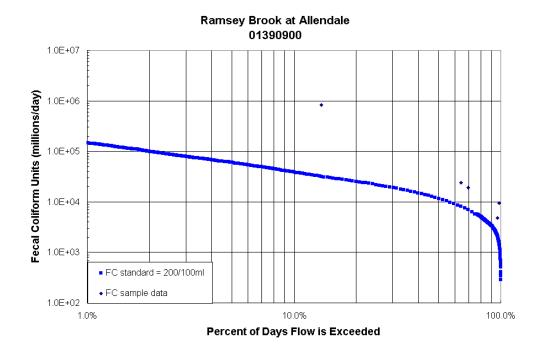
Load Duration Curve for Ramsey Brook at Allendale. Fecal coliform data from USGS station # 01390900 during the period 11/6/97 through 9/1/98. Water years 1970-2000 from USGS station # 01390500 (Saddle River at Ridgewood) were used in generating the FC standard curve.
