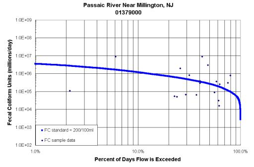
Load Duration Curve for the Passaic R Nr Millington. Fecal coliform data from USGS station # 01379000 during the period 10/1997 through 8/2000. Water years 1970-2000 from USGS station # 01379000 (Passaic R Nr Millington) were used in generating the FC standard curve.
