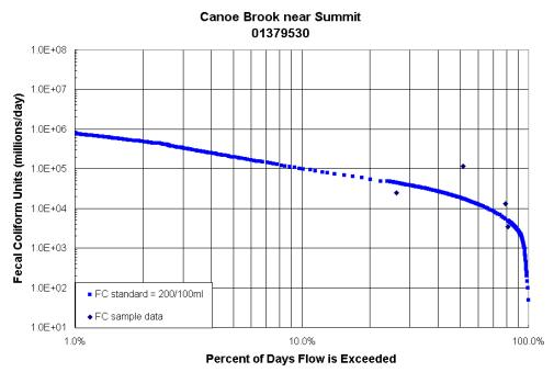
Load Duration Curve for Canoe Brook near Summit. Fecal coliform data from USGS station # 01379530 during the period 4/23/98 through 9/16/98. Water years 1970-2000 from USGS station # 01379530 (Canoe Brook near Summit) were used in generating the FC standard curve.
