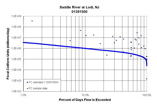
Load Duration Curve for Saddle River at Lodi. Fecal coliform data from USGS station # 01391500 during the period 2/22/94 through 9/13/00. Water years 1970-2000 from USGS station # 01391500 (Saddle River at Lodi) were used in generating the FC standard curve.
