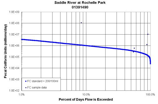
Load Duration Curve for Saddle River at Rochelle Park. Fecal coliform data from USGS station # 01391490 during the period 11/6/97 through 9/16/98. Water years 1970-2001 from USGS station # 01391500 (Saddle River at Lodi) were used in generating the FC standard curve.
