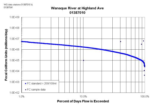
Load Duration Curve for Wanaque River at Highland Ave. Fecal coliform data from USGS station # 01387010 & 01387041 during the period 1/27/97 through 8/9/99. Water years 1970-2000 from USGS station # 01388500 (Pompton River at Pompton Plains NJ) were used in generating the FC standard curve.
