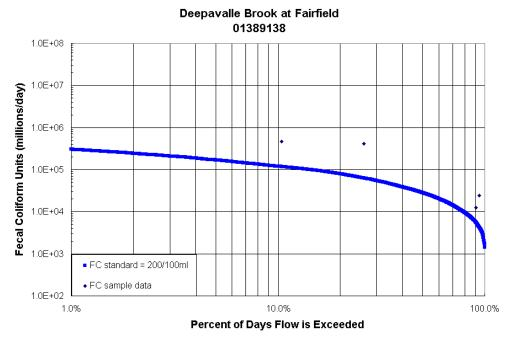
Load Duration Curve for Deepavalle Brook at Fairfield. Fecal coliform data from USGS station # 01389138 during the period 4/16/98 through 9/23/98. Water years 1970-2000 from USGS station # 01389500 (Passaic River at Little Falls) were used in generating the FC standard curve.
