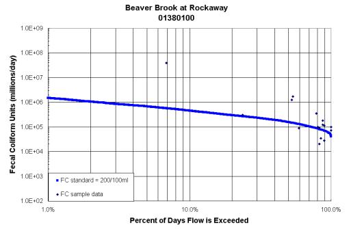
Load Duration Curve for the Beaver Brook At Rockaway. Fecal coliform data from USGS station # 01380100 during the period 11/13/97 through 8/7/2000. Water years 1970-2000 from USGS station # 01381500 (Whippany River at Morristown, NJ) were used in generating the FC standard curve.
