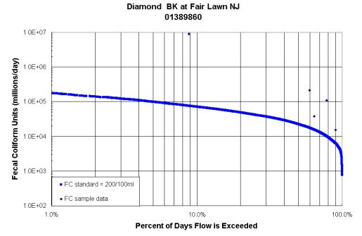
Load Duration Curve for Diamond Bk at Fair Lawn. Fecal coliform data from USGS station # 01389860 during the period 6/29/00-7/27/00. Water years 1970-2000 from USGS station # 01388500 (Pompton River at Pompton Plains NJ) were used in generating the FC standard curve
