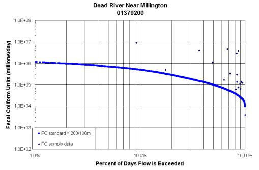
Load Duration Curve for the Dead River Near Millington. Fecal coliform data from USGS station # 01379200 during the period 10/1997 through 8/2000. Water years 1970-2000 from USGS station # 01379500 (Passaic R Nr Catham) were used in generating the FC standard curve.
