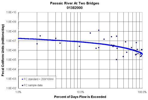
Load Duration Curve for the Passaic River at Two Bridges. Fecal coliform data from USGS station # 01382000 during the period 1/27/94 through 810/2000. Water years 1970-2000 from USGS station # 01381900 (Passaic R at Pine Brook, NJ) were used in generating the FC standard curve.
