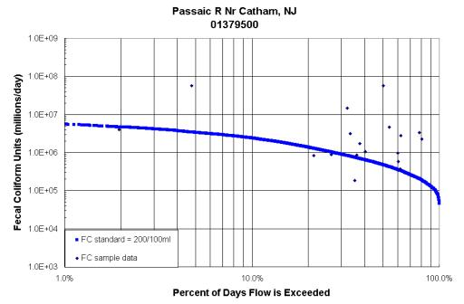
Load Duration Curve for the Passaic R Nr Catham. Fecal coliform data from USGS station # 01379500 during the period 10/1997 through 8/2000. Water years 1970-2000 from USGS station # 01379500 (Passaic R Nr Catham) were used in generating the FC standard curve.
