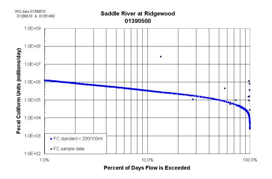
Load Duration Curve for Saddle R at Ridgwood. Fecal coliform data from USGS station # 01390510,01390518, & 01391490.during the period 11/6/97-8/9/99. Water years 1970-2001 from USGS station # 01390500 (Saddle River at Ridgewood) were used in generating the FC standard curve.
