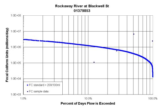
Load Duration Curve for Rockaway River at Berkshire Valley. Fecal coliform data from USGS station # 01379853 during the period 4/15/98 through 9/22/98. Water years 1970-2000 from USGS station # 01380500 (Rockaway River above Reservoir at Boonton) were used in generating the FC standard curve.
