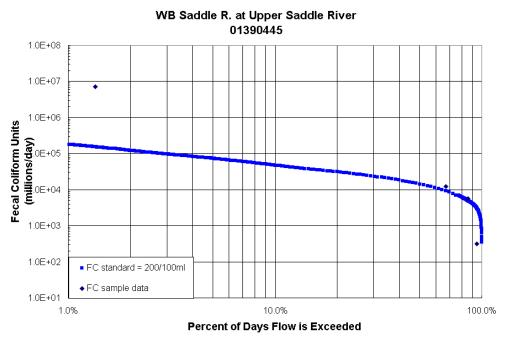
Load Duration Curve for WB Saddle R at Upper Saddle River. Fecal coliform data from USGS station # 01390445 during the period 11/4/99 through 8/7/00. Water years 1970-2001 from USGS station # 01390500 (Saddle River at Ridgewood) were used in generating the FC standard curve.
