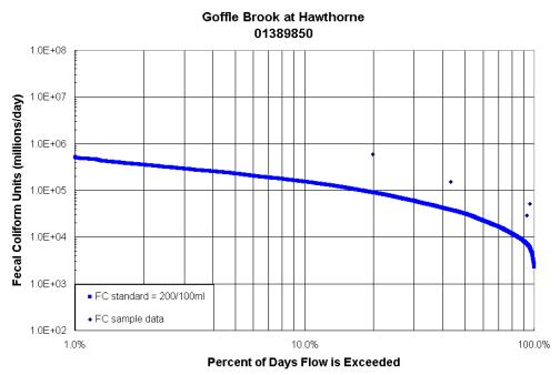
Load Duration Curve for Goffle Brook at Hawthorne. Fecal coliform data from USGS station # 01389850 during the period 4/23/98 through 9/24/98. Water years 1970-2000 from USGS station # 01388500 (Pompton River at Pompton Plains NJ) were used in generating the FC standard curve.
