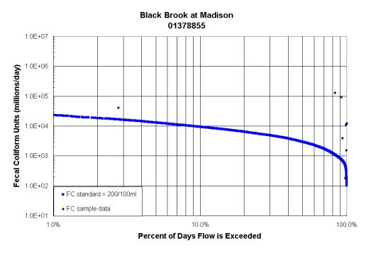
Load Duration Curve for Black Brook at Madison. Fecal coliform data from USGS station # 01378855 during the period 11/18/97 through 9/1/99. Water years 1970-2000 from USGS station # 01380500 (Rockaway River above Reservoir at Boonton) were used in generating the FC standard curve.
