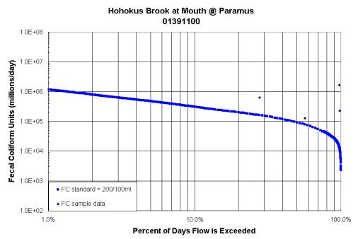
Load Duration Curve for Hohokus Brook at Mouth@ Paramus. Fecal coliform data from USGS station # 01391100 during the period 4/23/98 through 9/24/98. Water years 1970-2000 from USGS station # 01390500 (Saddle River at Ridgewood) were used in generating the FC standard curve.
