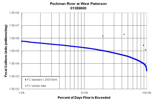
Load Duration Curve for Peckman River at West Patterson. Fecal coliform data from USGS station #01389600 during the period 4/23/98 through 9/24/98. Water years 1970-2000 from USGS station # 01388500 (Pompton River at Pompton Plains NJ) were used in generating the FC standard curve.
